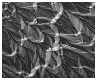
20nm layer of polycrystalline Co, Fresnel mode of Lorentz microscopy TEM (color represents direction), 200um, R. Dunin-Borkowski, Cambridge, 2004
