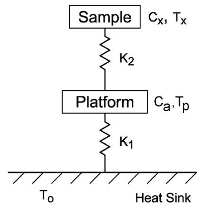
Fig. 1. Heat-flow diagram for a conventional thermal-relaxation calorimeter.
