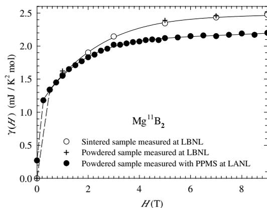
Fig. 7. The electron specific-heat for powdered  $\text{Mg}_{11}\text{B}_2$  as a function of magnetic field measured using the PPMS (●) are compared to those obtained using a custom-built, semi-adiabatic calorimeter at LBNL (○).
