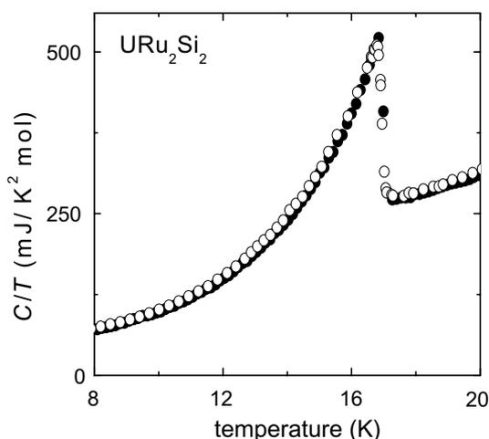
Fig. 5. A comparison of the specific-heat data of the PPMS (●) and a custom-built relaxation calorimeter (○) near the second-order transition in URu<sub>2</sub>Si<sub>2</sub>.
