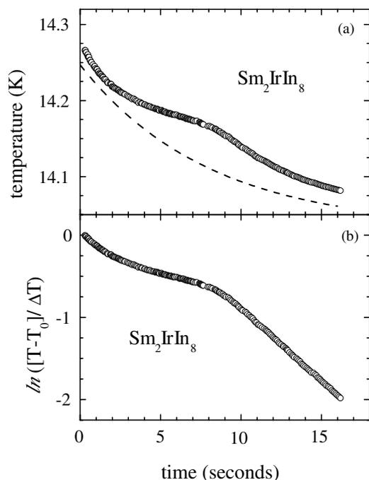
Fig. 9. (a) A plot showing the arrest in the temperature-time relaxation curve at the first-order transition in  $\text{Sm}_2\text{IrIn}_8$  near 14.18 K (points). The dashed line depicts an exponential-decay curve for comparison (the line is vertically offset for clarity). (b) Plot of thermal-relaxation decay data  $\ln[(T - T_0)/\Delta T]$  as a function of time that can be used to determine  $C_p(T)$  in the vicinity of a first-order transition.
