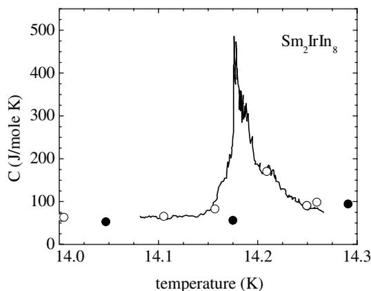
Fig. 10. Properly calculated specific-heat in the vicinity of the first-order transition at  $T_c = 14.18$  K in  $\text{Sm}_2\text{IrIn}_8$  (solid line). For comparison, time-constant fitting data for the custom-built calorimeter (O) and the PPMS curve-fitting data (●) are also presented in the figure.
