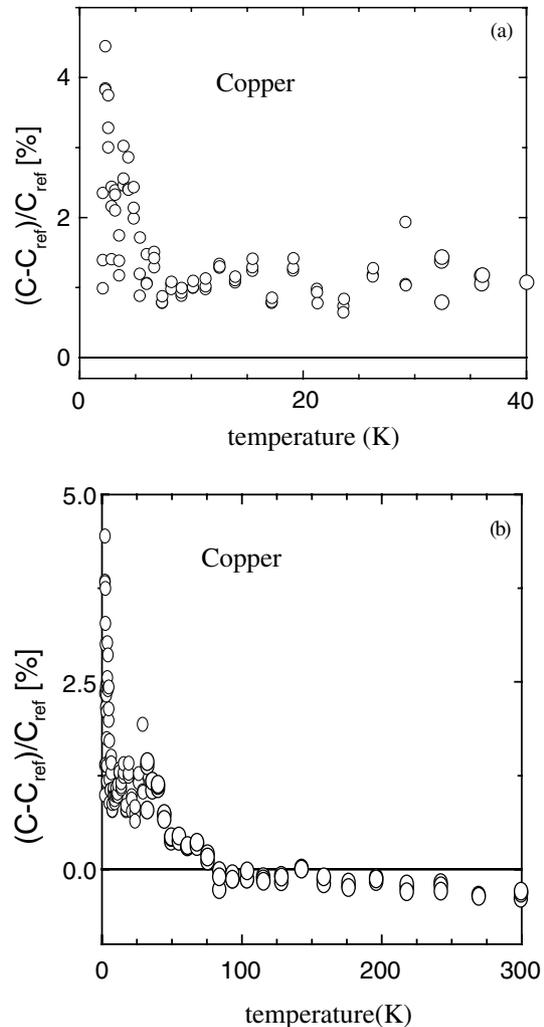
Fig. 2. A plot of the relative deviations from reference copper specific-heat data to that for the PPMS calorimeter at low temperatures (a) and to room temperature (b).
