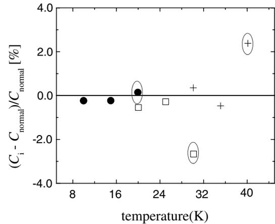
Fig. 3. The specific heat of copper measured after cooling slowly and after rapid cooling from room temperature at  $20 \text{ K min}^{-1}$ . After the measurements were made in the normal way the sample was cycled to room temperature. Following the rapid cooling from room temperature, three specific-heat points were measured on *cooling* from 20 to 10 K, 30 to 20 K, and 40 to 30 K. The first point measured in each series is circled.
