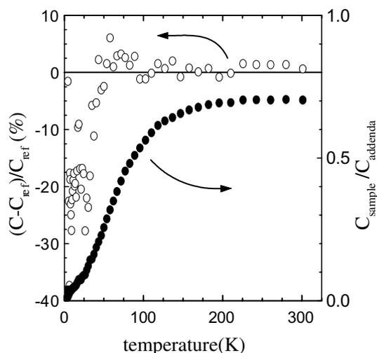
Fig. 4. A plot of the relative deviations of the PPMS sapphire results from the reference specific-heat data [22].
