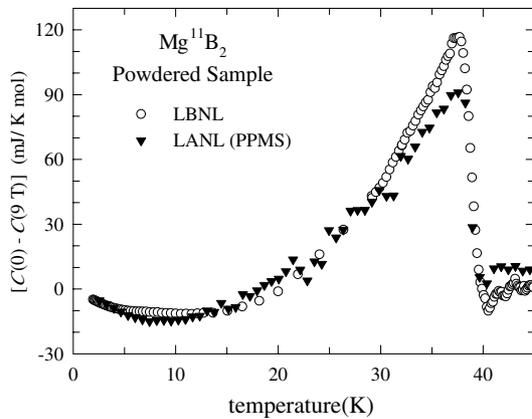
Fig. 6. A comparison of the specific-heat data of the PPMS and a custom-built semi-adiabatic calorimeter at LBNL at the critical temperature for the superconductor  $\text{Mg}_{11}\text{B}_2$ .
