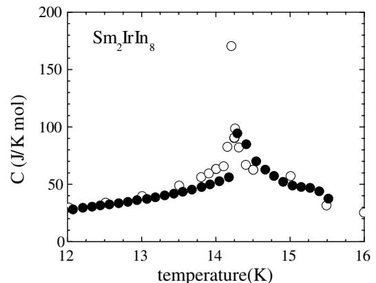
Fig. 8. A comparison of the specific-heat data from the PPMS (●) with that from a custom-built relaxation calorimeter (○) near the first-order transition in  $\text{Sm}_2\text{IrIn}_8$ .
